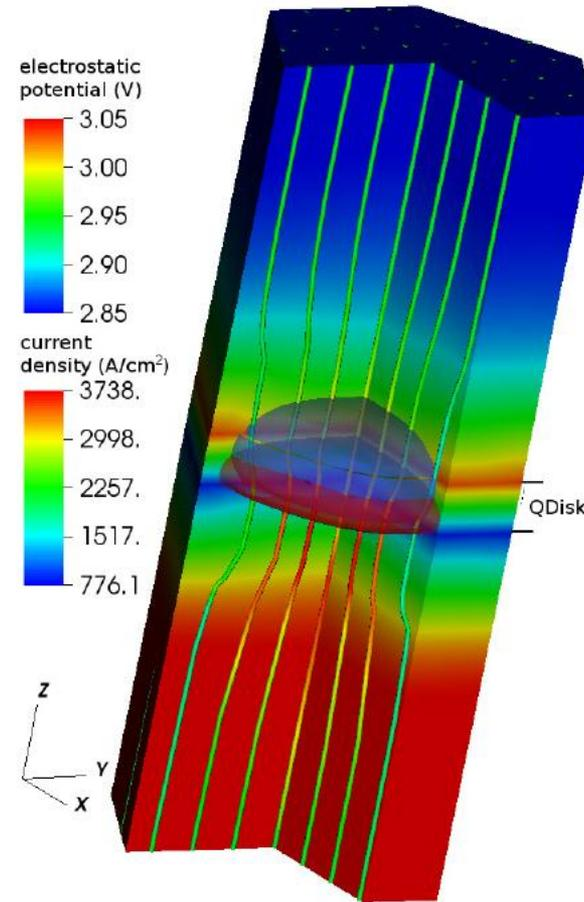
*The electrostatic potential and current flow lines around the intrinsic part of the column. Classical and quantum results. The selfconsistent EFA/ETB/drift-diff. results shows also the contours of the electron and hole densities at half of the mean density inside the intrinsic region.*
