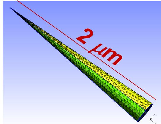
Here the STM tip and the probed molecule and substrated is modelled by using a multiscale FEM/atomistic approach
