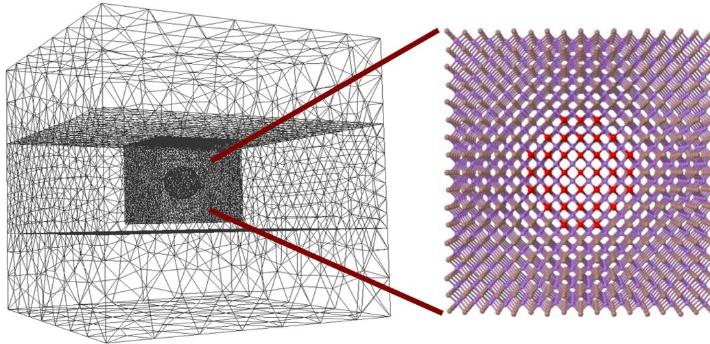
Now atomistic structure is only defined in a smaller box (4nm) with 4000 atoms
