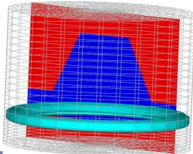
Spatial separation of electrons and holes mainly due to electric polarization
