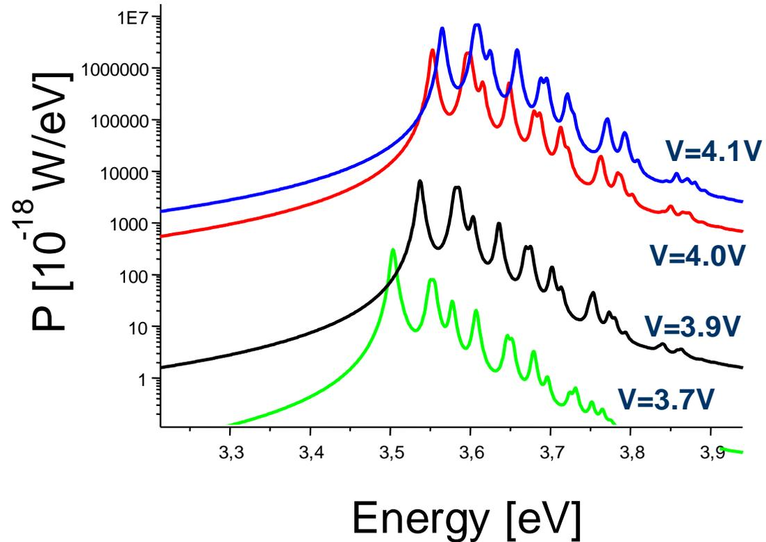
A 0.5 eV blue shift of the fundamental emission peak is obtained going from 3.7V (below threshold) to 4.1 (above threshold) due to the combined effect of polarization and screening .
